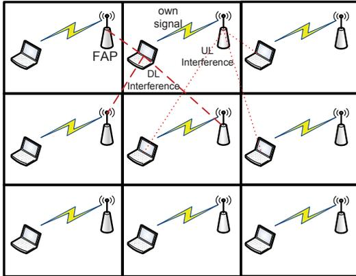
Fig. 7.3 Intercell interference in the uplink and downlink.
