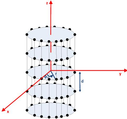
Fig. 2. Cylindrical array.
