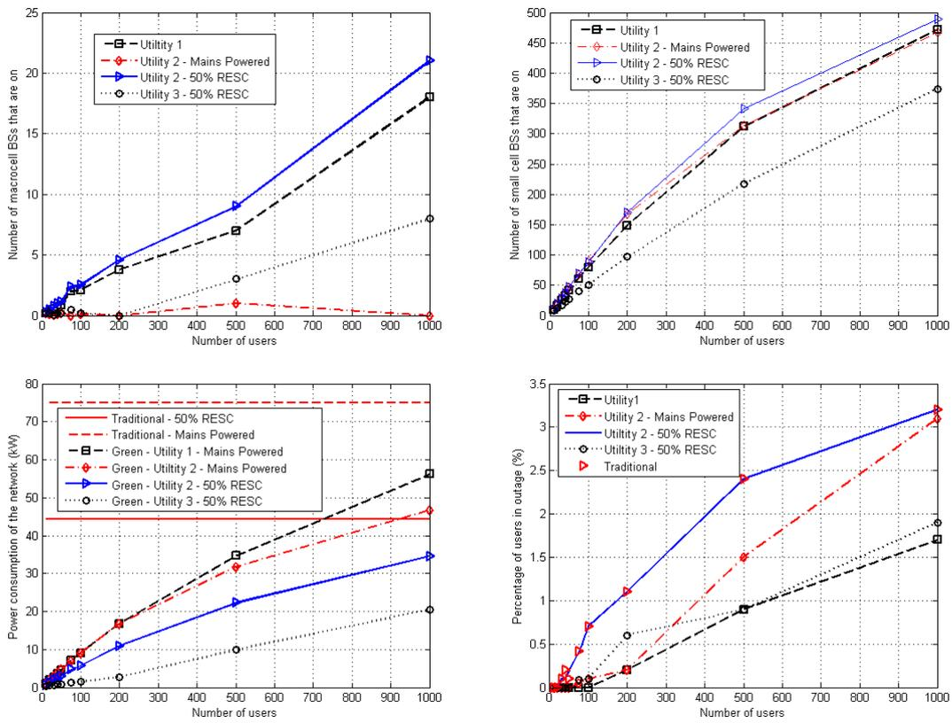
Fig. 5. Performance results for Service 4. Upper Left: Number of macrocell BSs switched on. Upper Right: Number of small cell BSs switched on. Bottom Left: Network power consumption. Bottom Right: Percentage of users in outage.
