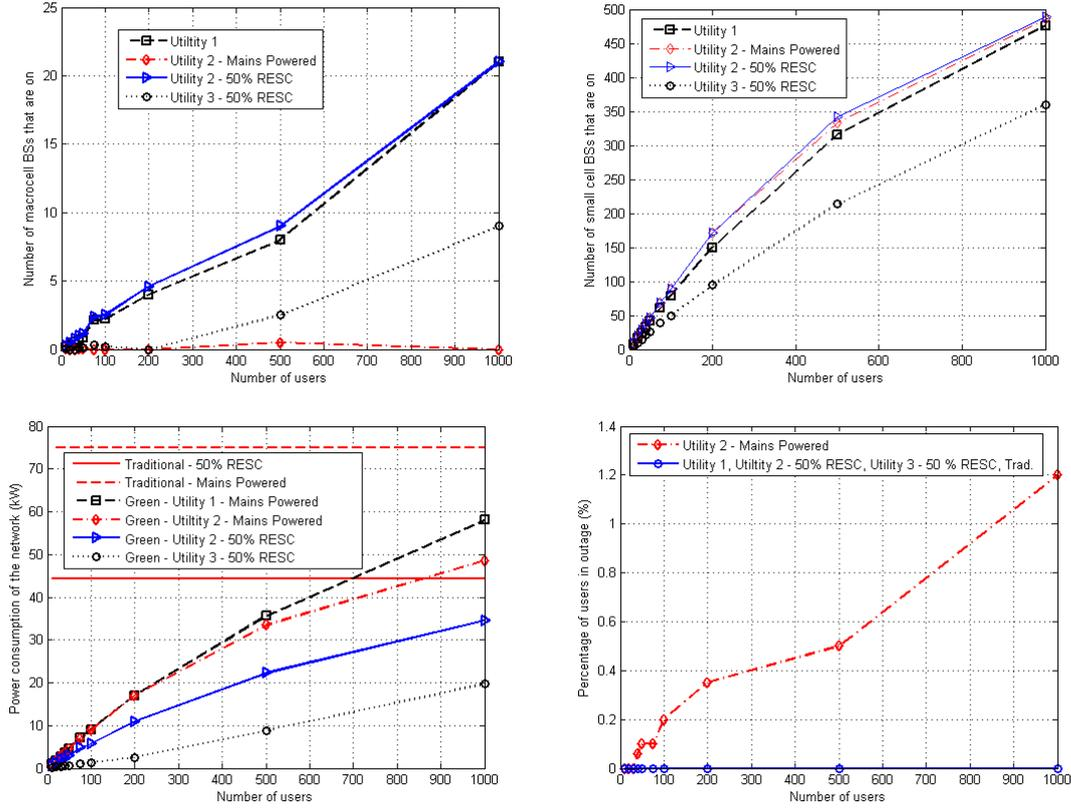
Fig. 2. Performance results for Service 1. Upper Left: Number of macrocell BSs switched on. Upper Right: Number of small cell BSs switched on. Bottom Left: Network power consumption. Bottom Right: Percentage of users in outage.
