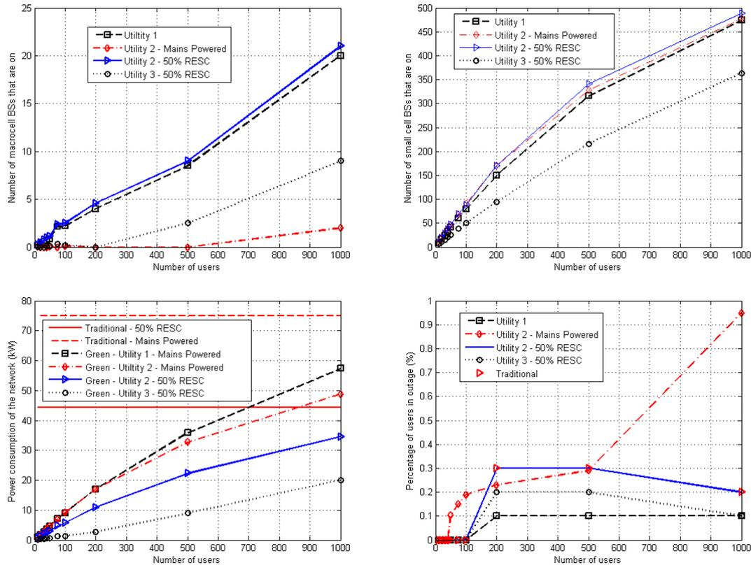
Fig. 4. Performance results for Service 3. Upper Left: Number of macrocell BSs switched on. Upper Right: Number of small cell BSs switched on. Bottom Left: Network power consumption. Bottom Right: Percentage of users in outage.
