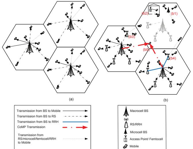
Fig. 1. Network Example: (a) Macrocell only. (b): Green heterogeneous network.
