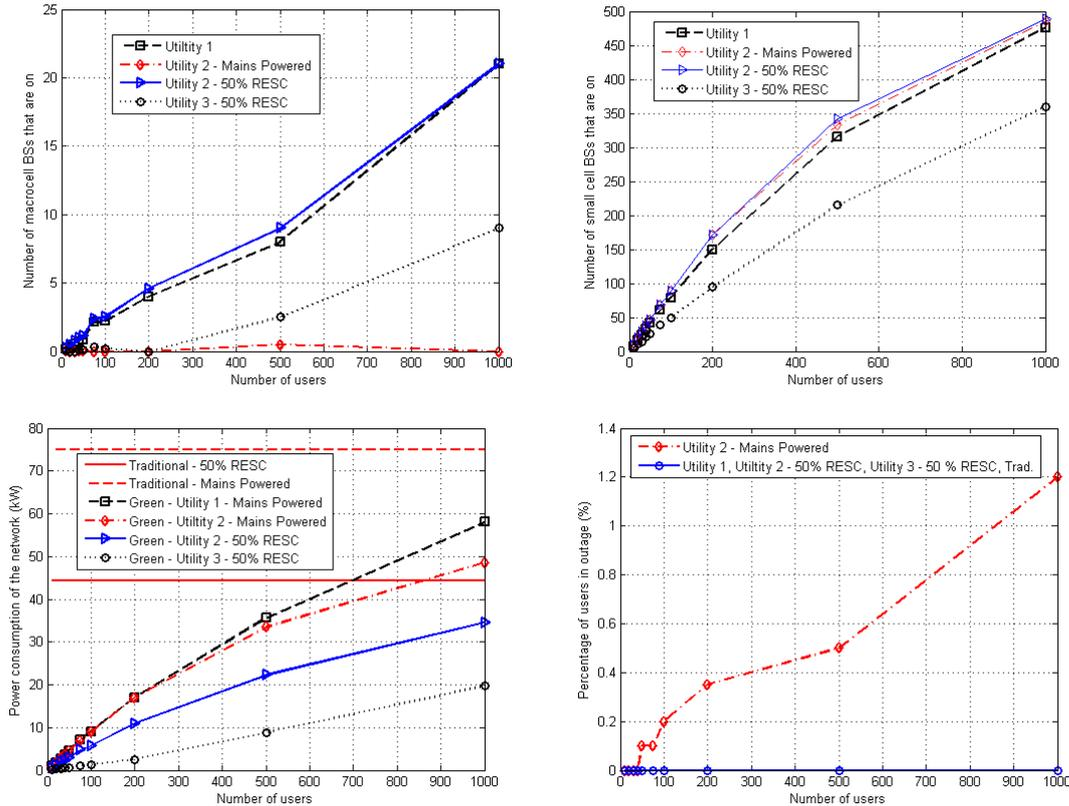
Fig. 3. Performance results for Service 2. Upper Left: Number of macrocell BSs switched on. Upper Right: Number of small cell BSs switched on. Bottom Left: Network power consumption. Bottom Right: Percentage of users in outage.
