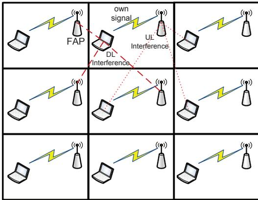
Fig. 2 Intercell interference in the uplink and downlink.
