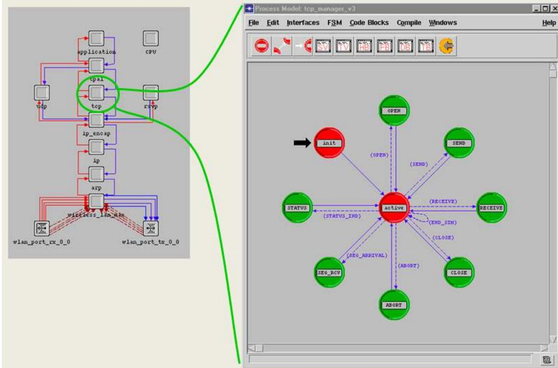
Figure 4. An example of Process domain in OPNET
