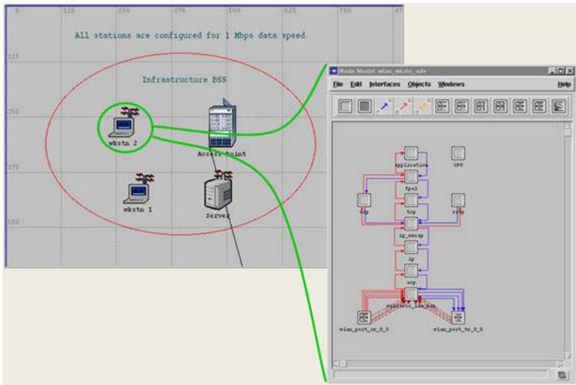
Figure 3. An example of Node domain in OPNET
